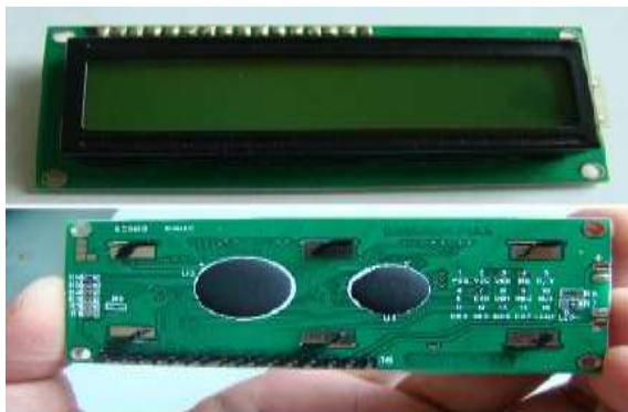
16-pin LCD, Pin 15 Led+ and Pin 16 is LED-
